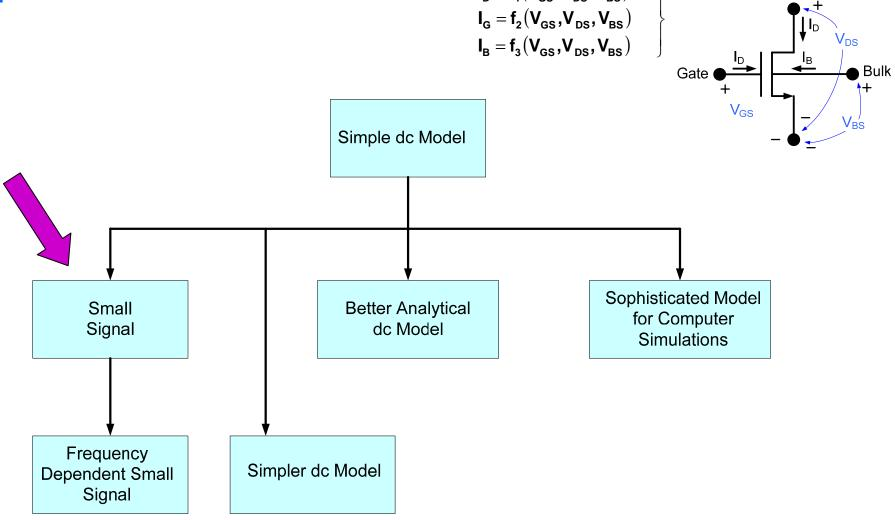
Goal with small signal model is to predict performance of circuit or device in the vicinity of an operating point
