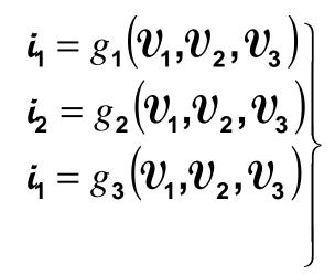
Small signal model is that which represents the relationship between the small signal voltages and the small signal currents
