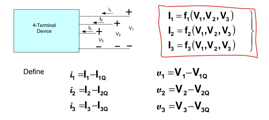
Small signal model is that which represents the relationship between the small signal voltages and the small signal currents
