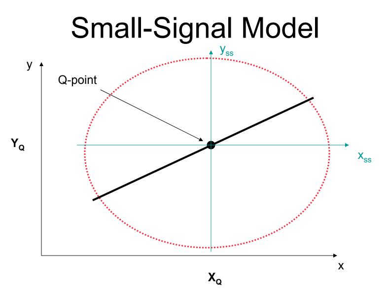
Device Behaves Linearly in Neighborhood of Q-Point Can be characterized in terms of a small-signal coordinate system
