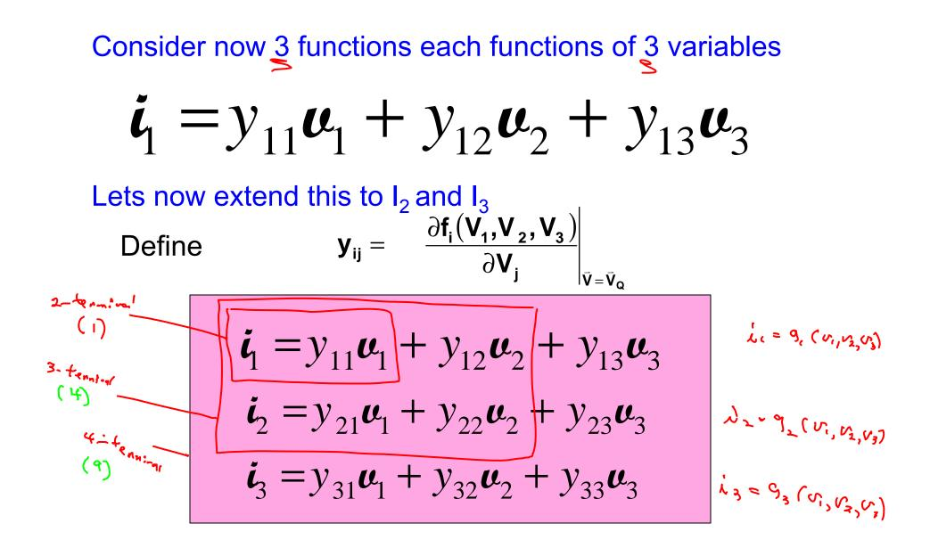
This is a small-signal model of a 4-terminal network and it is linear
